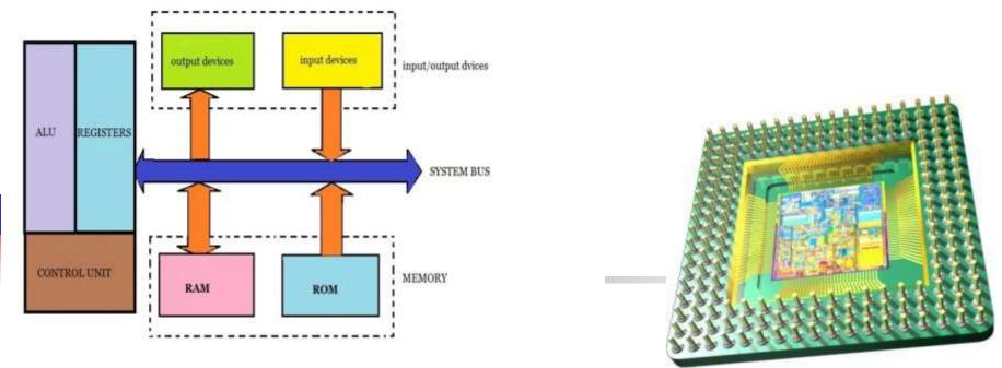
The microprocessor is a multipurpose, <u>programmable</u> device that accepts <u>digital data</u> as input, processes it according to instructions stored in its memory, and provides results as output. Medha Excitation & Propulsion Control System - MEP-660
