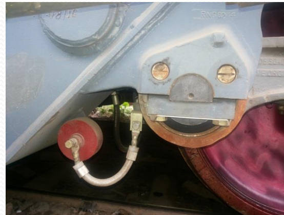
Resistor earthing cable
