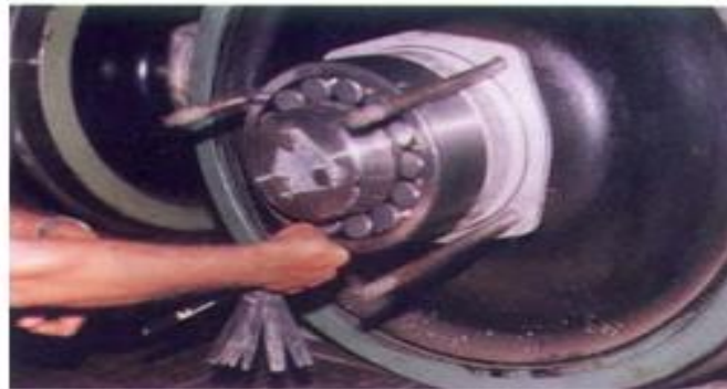
Fig: 3.0 Checking Bearing radial clearance in mounted condition
