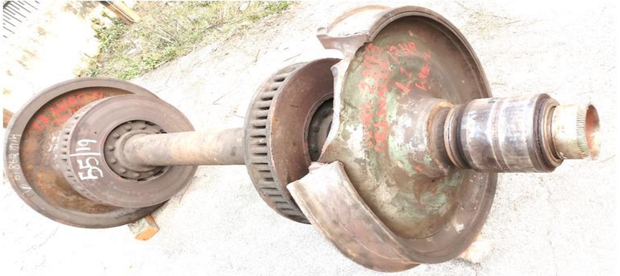
Fig.1: Photograph showing fractured wheel set in as received condition.
