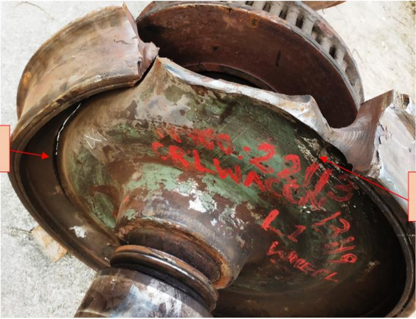
Fig.4: Photograph showing two numbers of crack in fractured wheel set.
