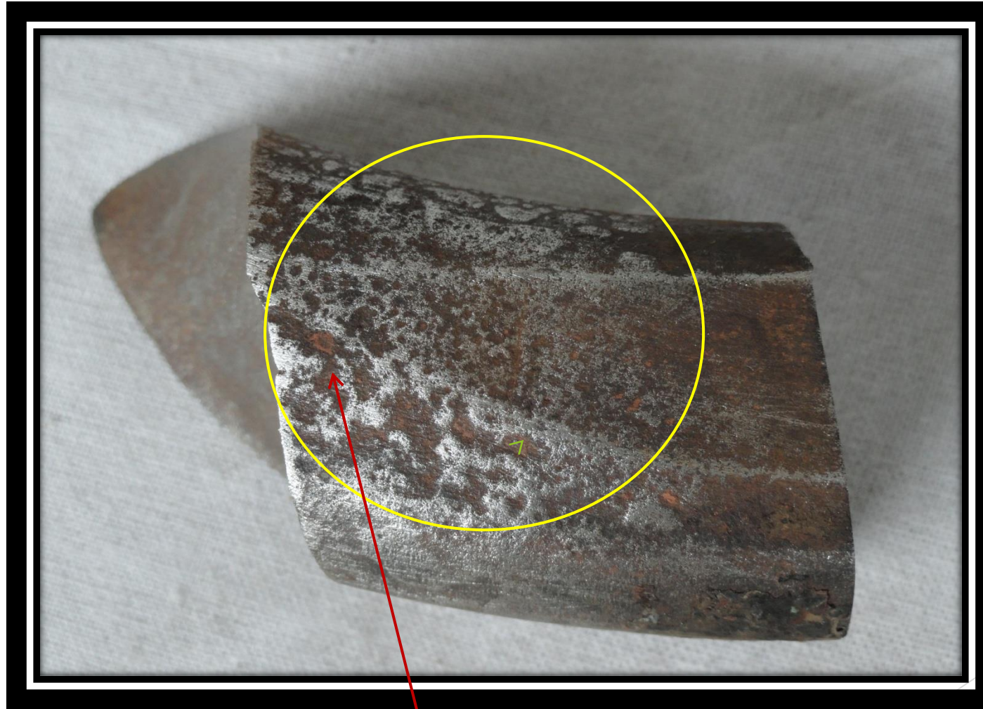
Areas showing deep corrosion pits
