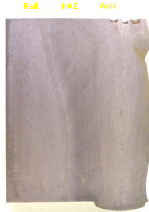
Fig.7: Photograph showing weld, heat affected zone & parent metal of sample no 76/2022.
