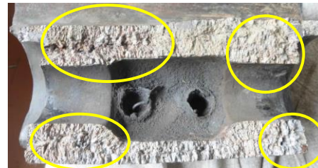
Fig.2:-Fracture Face of broken knuckle showing presence of shrinkage cavities, porosities.
