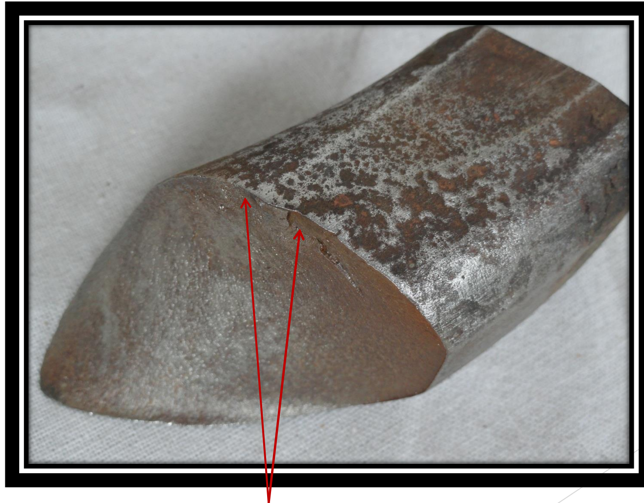
Arrows indicate the corrosion pits as points of stress concentration and nuclei of fatigue causing failure
