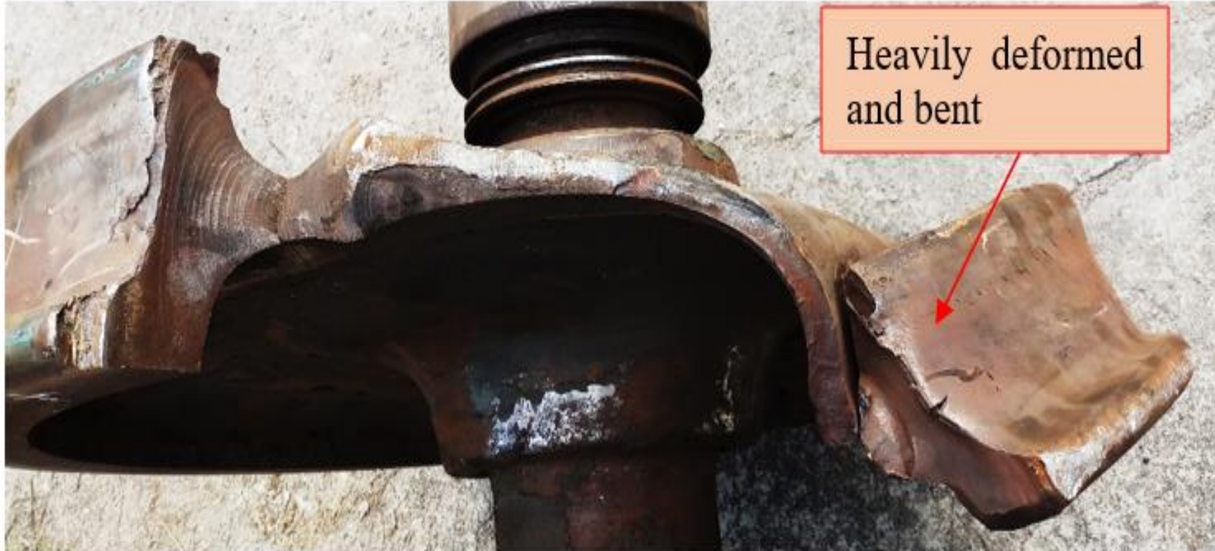
Fig.5: Photograph showing fracture face of the wheel set.
