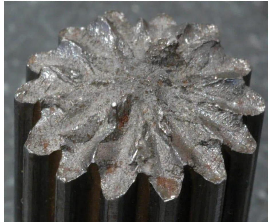
Failure of a splined shaft
