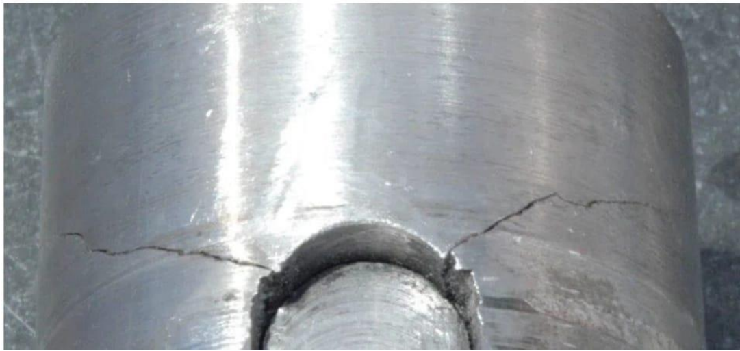
Two 45° cracks started at the keyway
