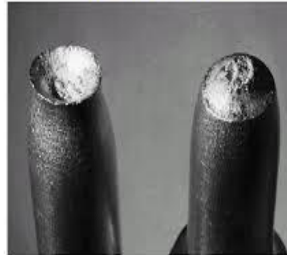
(Cup-and-cone fracture in Al)
