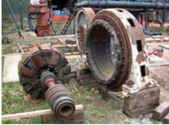
The rotor and stator of 3-phase generator
