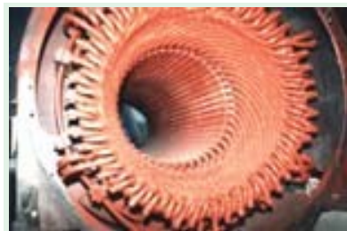
Windings of induction electric motor
