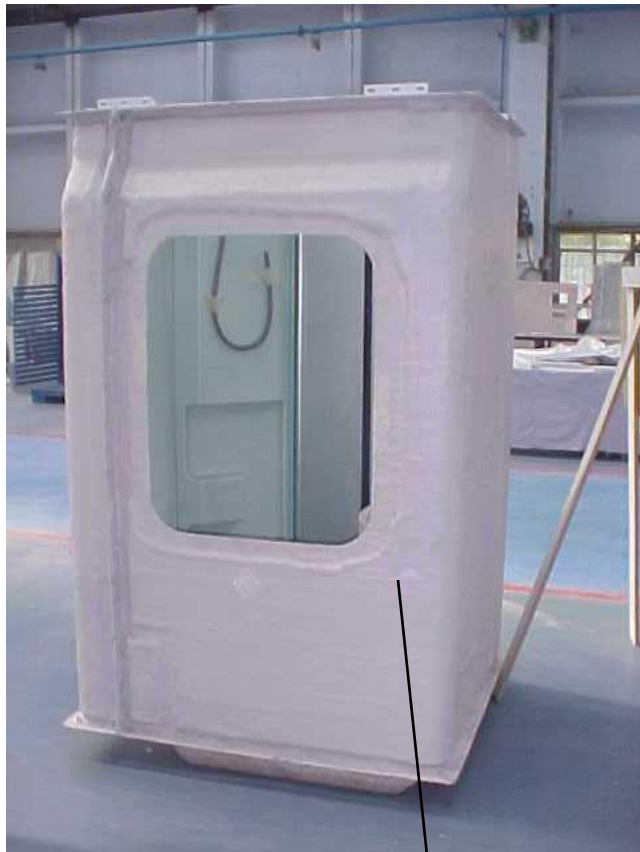
FRP LAVATORY MODULE (PVC FOAM SANDWICHED BETWEEN FRP)
