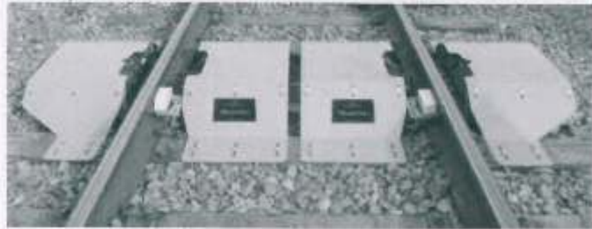
Wheel Profile Measuring System for wheel defects like sharp flange root wear etc
