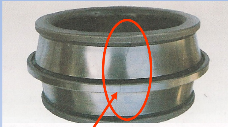
Inner race Crack
