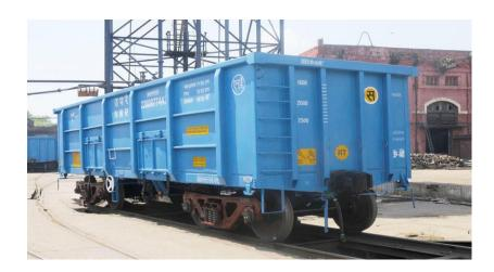
This bogie open wagon was designed in year 2005, 250 mm longer, 76 mm higher and 50 mm wider than BOXN and BOXNHS wagon at 22.9 t axle load. The wagon is manufactured by using stainless steel and cold rolled sections. Air-braked, CBC couplers, roller bearings.
