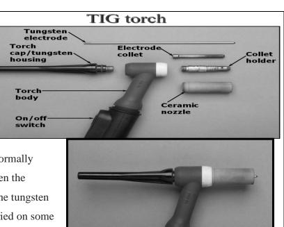
operations (up to about 200 A), while water cooling is required for high-current welding (up to about 600 A). The torches are connected with cables to the power supply and with hoses to the shielding gas source and where used, the water supply.
