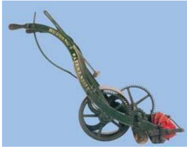
Lawn-mover is a combination of kinematic links.
