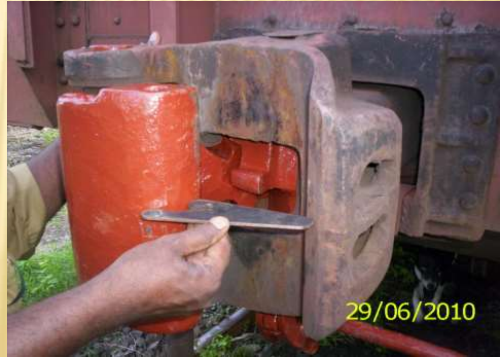
Wrong practice of gauging
