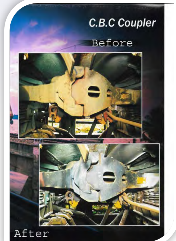
BEFORE AND AFTER IMAGES OF C.B.C.COUPLER
