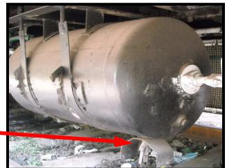
**If brakes are released, close the isolation cocks of both brake cylinders and work the train.**
