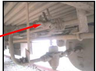
**Isolate DV by lifting isolating handle and again pull the release lever of DV.**
