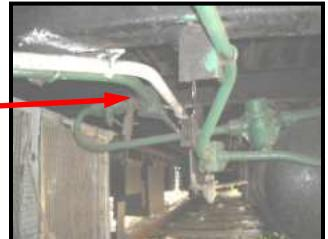
**Check that brakes are released by shaking the brake blocks.**
