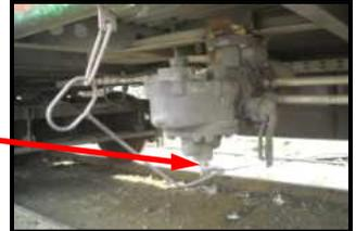
**Isolate FP and BP branch pipe and drain AR.**
