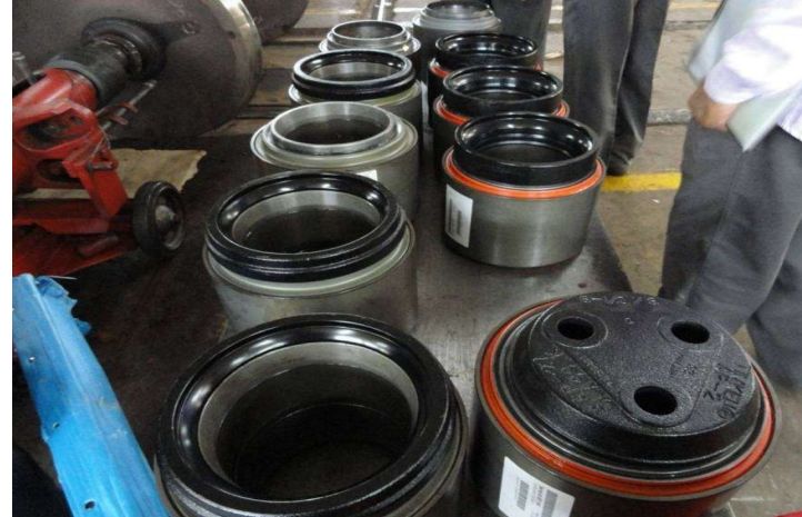
Bearings stored in dry place
