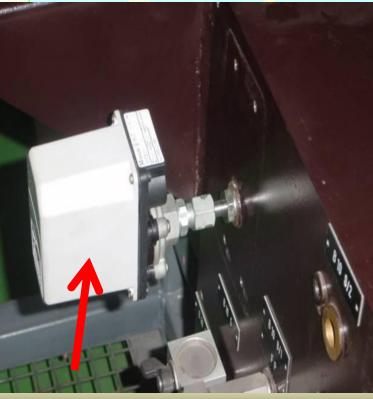
**Testing procedure (Faiveley)** Step 1: Diagnostic of Faults As push button 1 is pushed & Ð the code displayed is different to 99 (i.e. 95 or 72 or 73) or the system is switched off. The CPU Pushbutton : will switch on & by pressing the push button 1 for minimum 3sec, the faults can be displayed. The following functions also take place: Indication "88" for 3 sec (7-segment LED test) Indication of all faults in a sequence of 3 sec.
