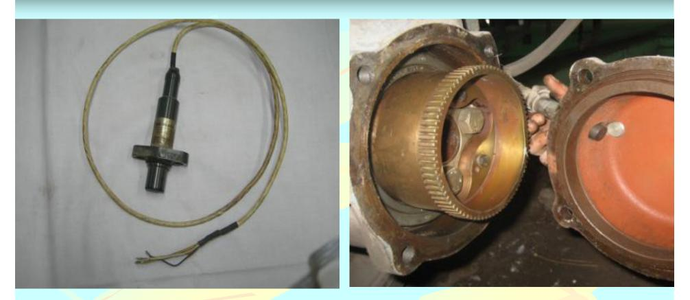
The air gap between the rotating gear (Phonic wheel) & speed sensors probe should be Knorr Bremse = 0.4 to 1.4 mm Faiveley = 1.5 ± 0.5 mm
