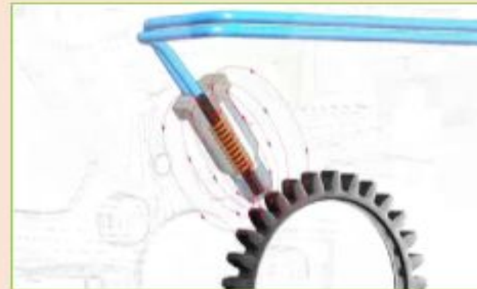
Pics. Showing change in internal inductance of the adjacent sensor
