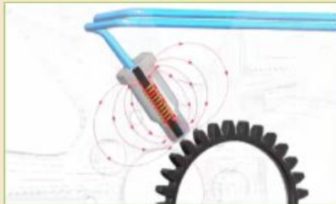
Pics. Showing change in internal inductance of the adjacent sensor
