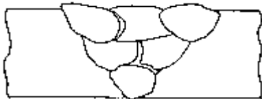
lack of fusion between passes
