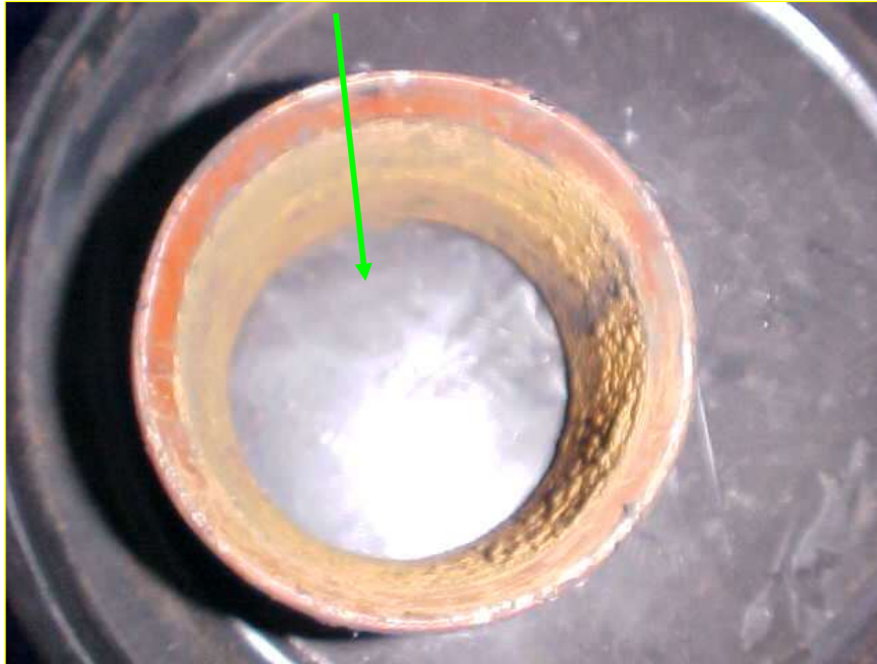
Corroded inner layer of dresser joint of WDS6 locomotive
