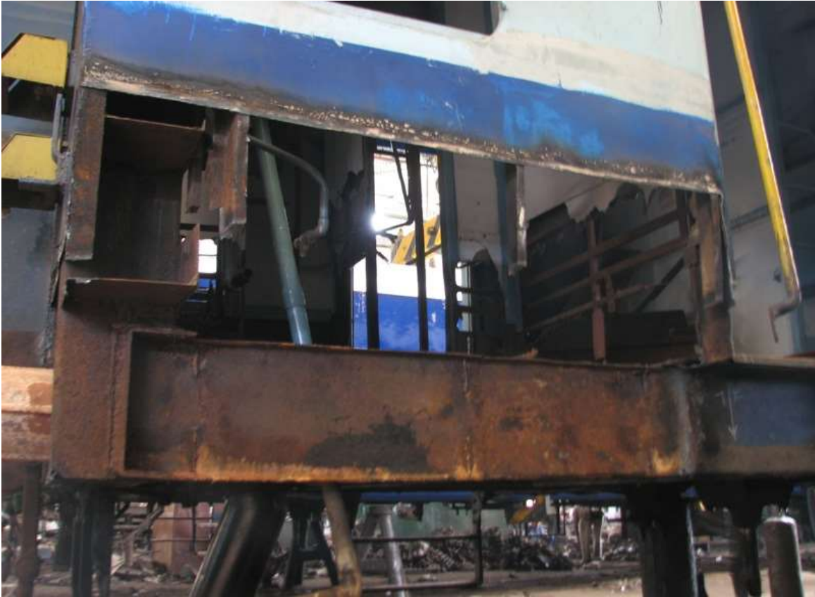
Corroded Sole Bar & Lavatory
