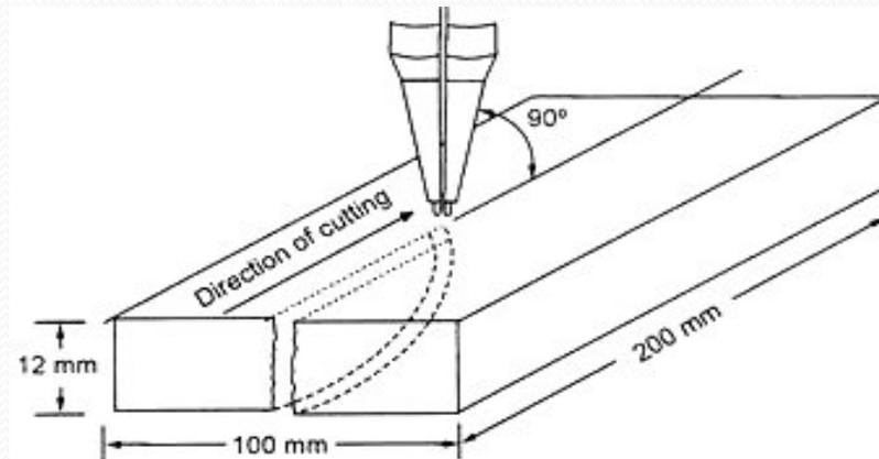
Fig. 7.1(A) M.S. Plate Cutting Procedure
