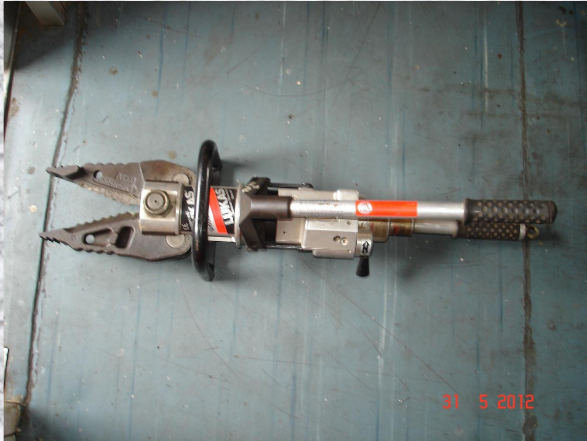
Hand operated combined Cutter and Spreader with built in Pump
