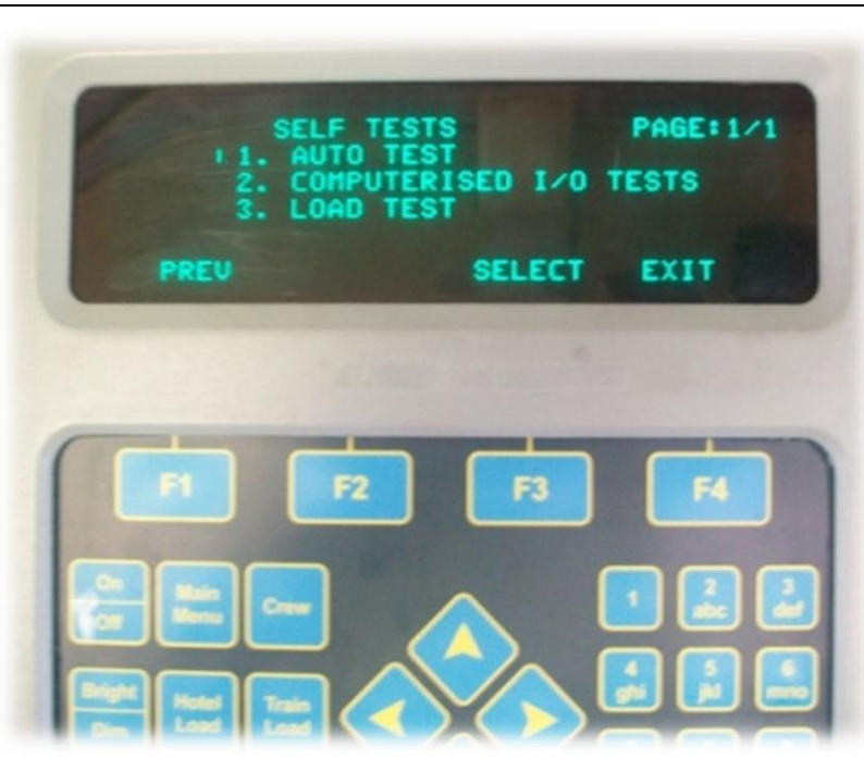
Bring cursor to AUTO TEST and press F3 or press numeric key 1. Fig. 3.21
