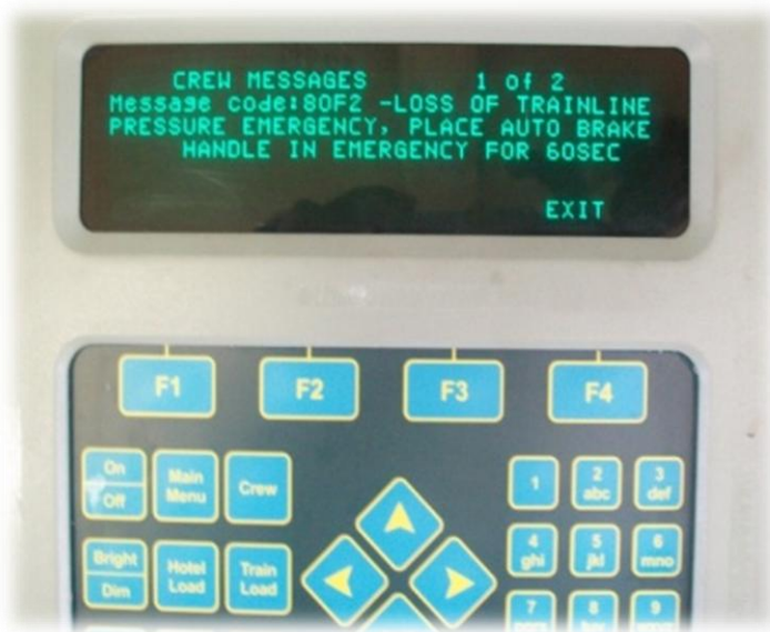
In Crew Message, 'LOSS OF TRAIN LINE PRESSURE EMERGENCY, PLACE AUTO BRAKE IN EMERGENCY FOR 60 SEC'. Keep Auto Brake in emergency for 60 seconds. Fig. 3.26
