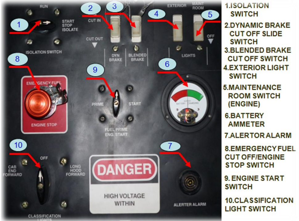
Fig. 1.13 ENGINE CONTROL PANEL (ECP) IN MEDHA DUAL CAB LOCO
