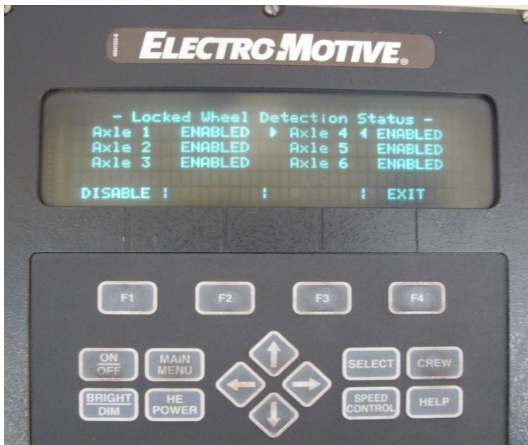
Move cursor by navigation keys to defective sensor axle and press F1. Fig. 5.29
