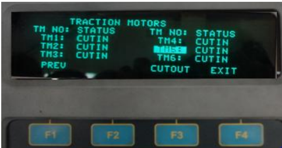
Bring cursor to defective TM by using arrow keys and press F3 to cut out. Fig. 5.8
