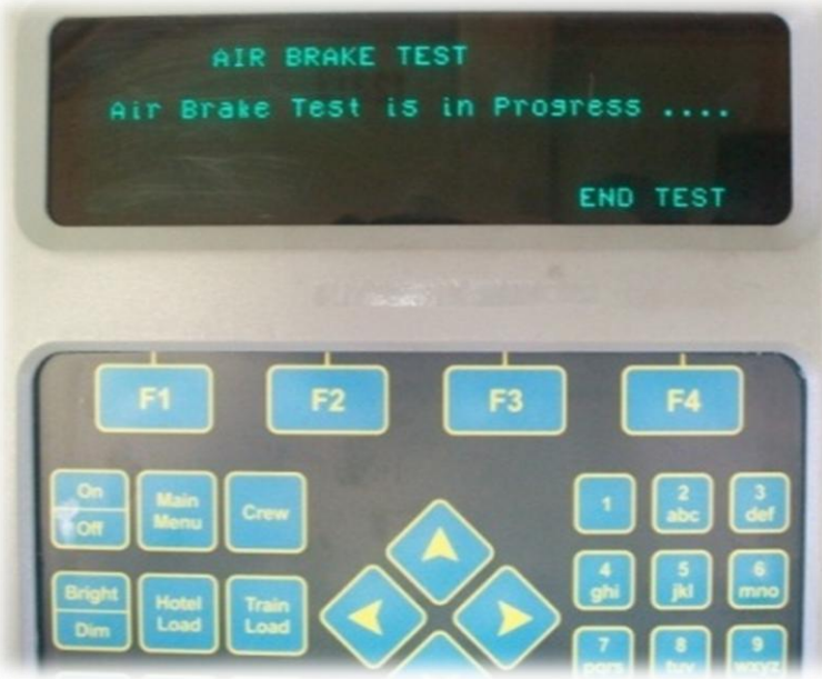
Air Brake Test is in Progress. Fig. 3.24 (Do not disturb any handle positions).
