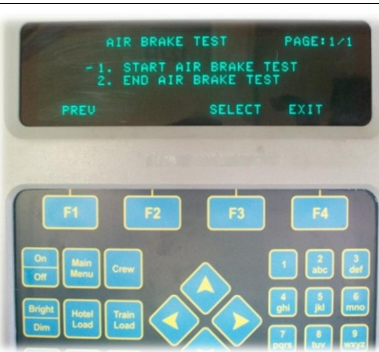
Bring cursor to START AIR BRAKE TEST and press F3 or press numeric key 1. Fig. 3.23
