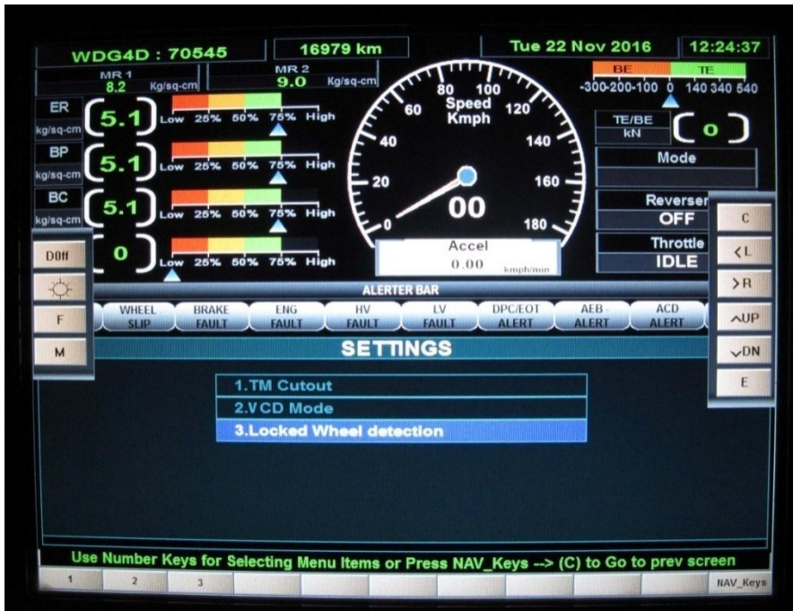
On right side pop up menu touch UP/DN keys to select Locked Wheel detection and Touch 'E' Key or Touch No. '3' Key. Fig. 5.45
