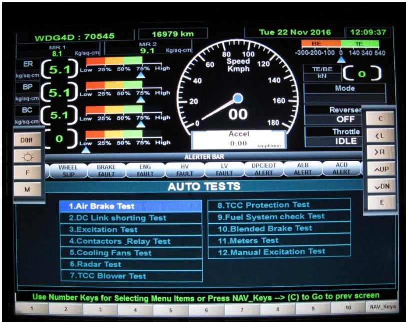
Auto Tests Screen appears. On right side pop up menu touch UP/DN keys to select Air Brake Tests and Touch ' E ' Key or Touch No. ' 1 ' Key. Fig. 3.43
