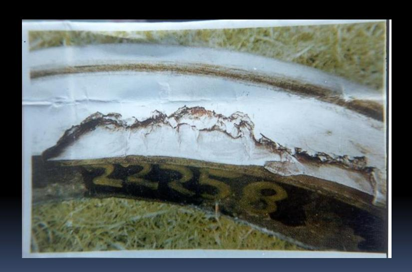
Spread Rim; If the rim widens out for a short distance on the front face, aninternal defect may be present. Spreading of the rim is usuallyaccompanied by a flattening of the tread, which may or may nothave cracks or shelling on the tread. Such wheels must be withdrawn from service.(This condition should not be confused with a uniform curling overof the outer edge of the rim around the entire wheel, which is called rim flow. Rim flow is not a rejectable defect).
