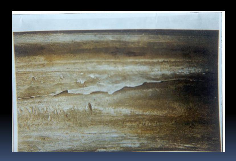
Shelled Tread; Shelling can be identified by pieces of metal breaking out of thetread surface in several places more or less continuously around therim. Shelling takes place when small pieces of metal break out between the fine thermal checks. These aregenerally associated with small skid marks or "chain sliding" Suchwheelsshould bewithdrawn from service and sent to workshops for re-profiling.
