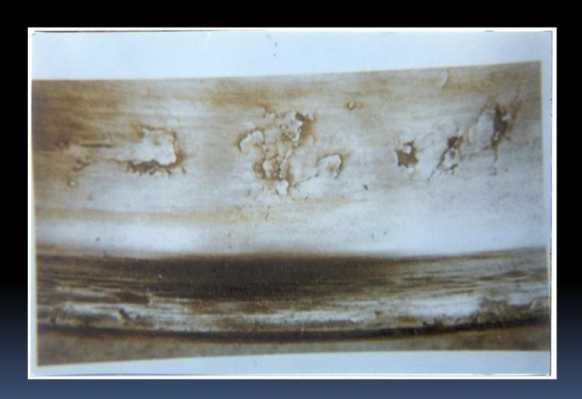
Thermal Cracks; Thermal cracks appear on a wheel tread due to intense heating of the wheel arising out of severe brake binding. Such cracks occur on the tread and generally progress across the tread in a transverse & radial direction. Whenever suchacrack becomes visible on the outer face of the rim or tread crack has reached the outer edge(non-gauge face) of the rim, the wheel should be withdrawn from service.
