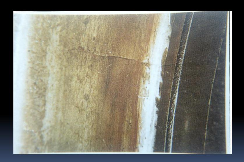
If a crack becomes visible on the outer flange face, thewheel should be withdrawn from service. Such wheels should be sent to workshop for examination and subsequent rejection. Wheels involved in brake binding during service, should be examined carefully during the maintenance to rule out thepossibility of rejectable thermal cracks. Such wheels may be identified by presence of flats (even within acceptable limits) and severe discoloration or blue/ black heating marks on the tread
